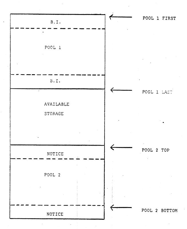
Fig. 1. Core Storage Layout during program execution.
